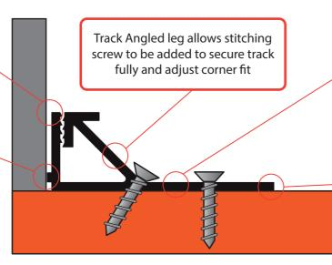
The extra wide track allows the use of Automatic Collated screw guns to be used for the quickest installation
