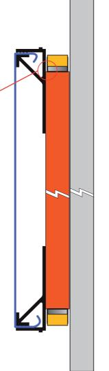
One track for all applications! The use of a thicker outside leg allows the track to function as both a perimeter AND intermediate track
